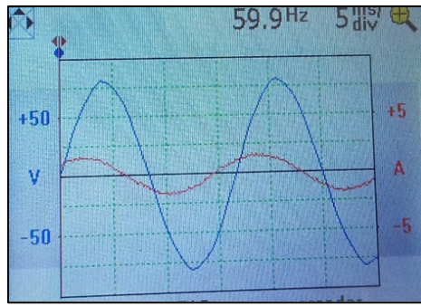
Fig. 5: Voltage and current waveform for the engine with load.
